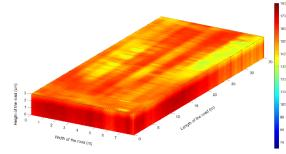
Figure 1. 3D asphalt temperature profile
