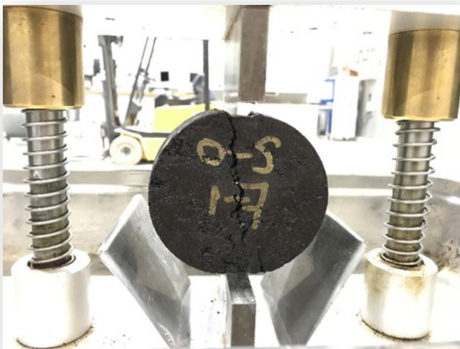
ITSR being performed on an AC11 surf sample at AKC
