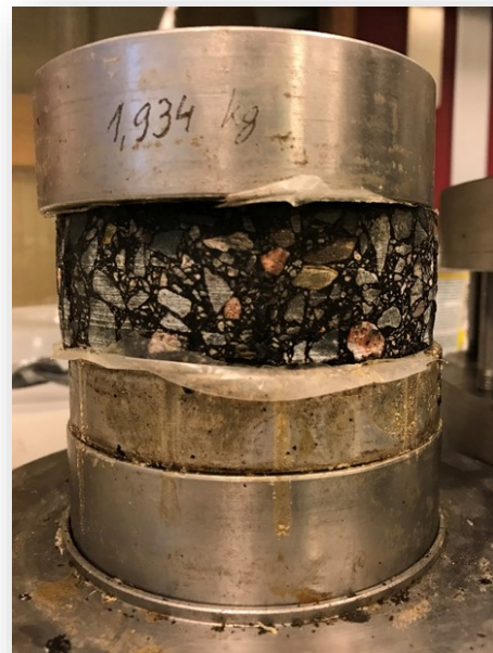
AC11 surf sample after Triaxial CC test
