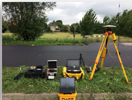
Off-the-shelf components of the Real-time Process Control System developed by Denis Makarov: On-board tablet to show Visuals in real time (left), Cooling Curve Calibration unit (middle), Vodafone Wi-Fi router and Trimble GPS receiver (far right)
