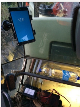
Off-the-shelf components of the Real-time Process Control System developed by Denis Makarov: On-board tablet to show Visuals in real time (left), Cooling Curve Calibration unit (middle), Vodafone Wi-Fi router and Trimble GPS receiver (far right)
