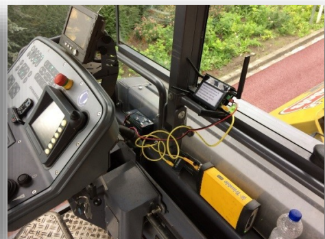
Off-the-shelf components of the Real-time Process Control System developed by Denis Makarov: On-board tablet to show Visuals in real time (left), Cooling Curve Calibration unit (middle), Vodafone Wi-Fi router and Trimble GPS receiver (far right)
